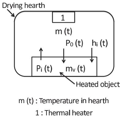
Fig. 1: Static model in the drying oven
