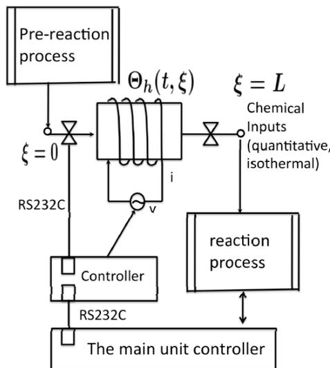
FIGURE 14. Reaction process control system equipment
