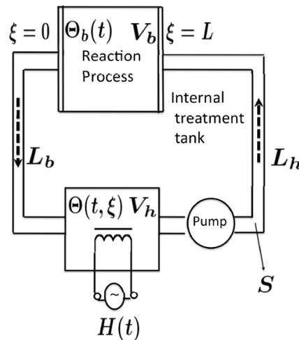
FIGURE 8. System model of the external heat system
