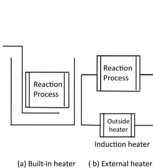
FIGURE 5. (a) Built-in heater, (b) outside heater
