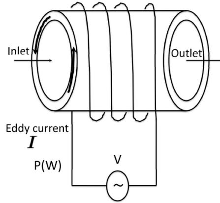
FIGURE 11. Schematic of the induction heating
