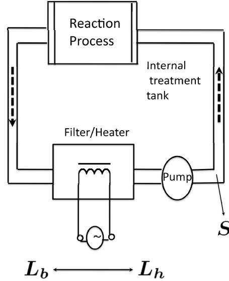
FIGURE 6. Detailed model of AEHE
