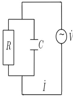
FIGURE 12. The equivalent circuit of the induction heating
